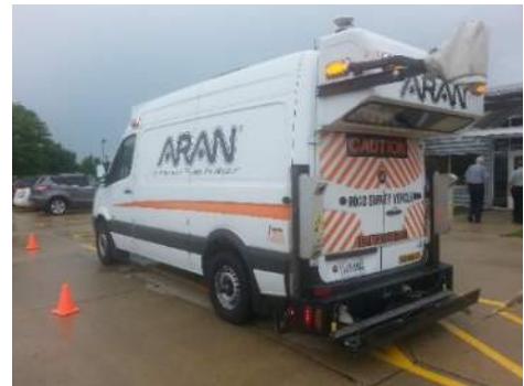
Figure 12 – Automatic Data Collection Vehicle
