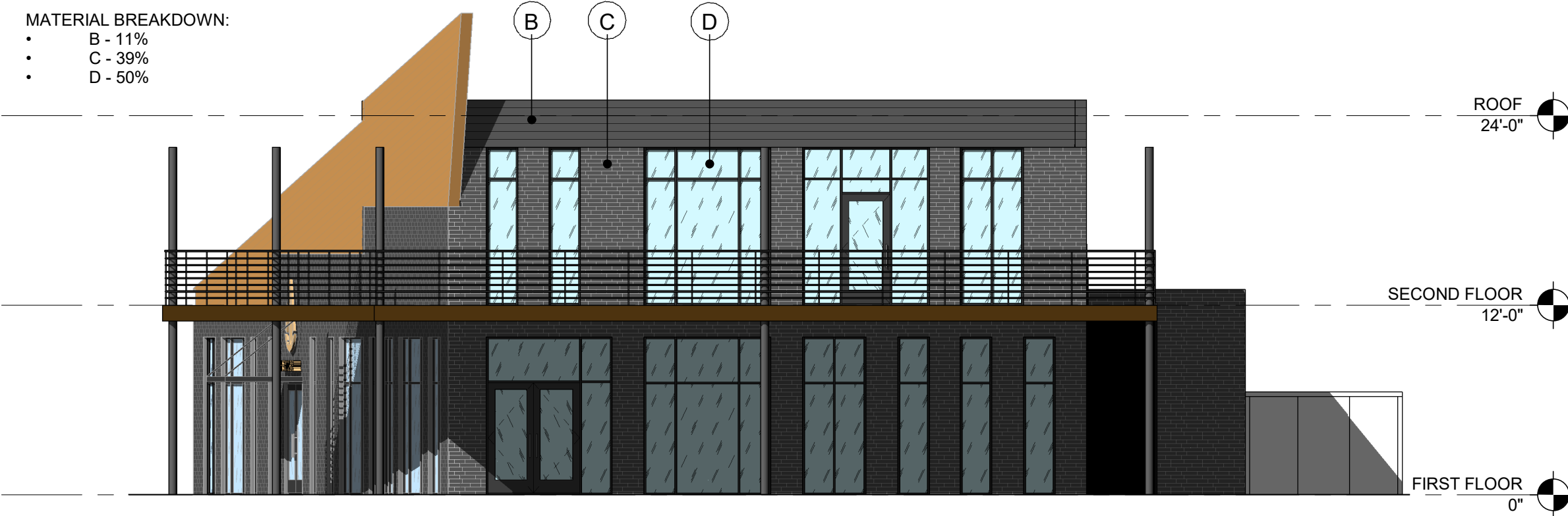
A2 SOUTH ELEVATION SCALE: 1/8" = 1'-0" MIN 70% PRIMARY MATERIALS
