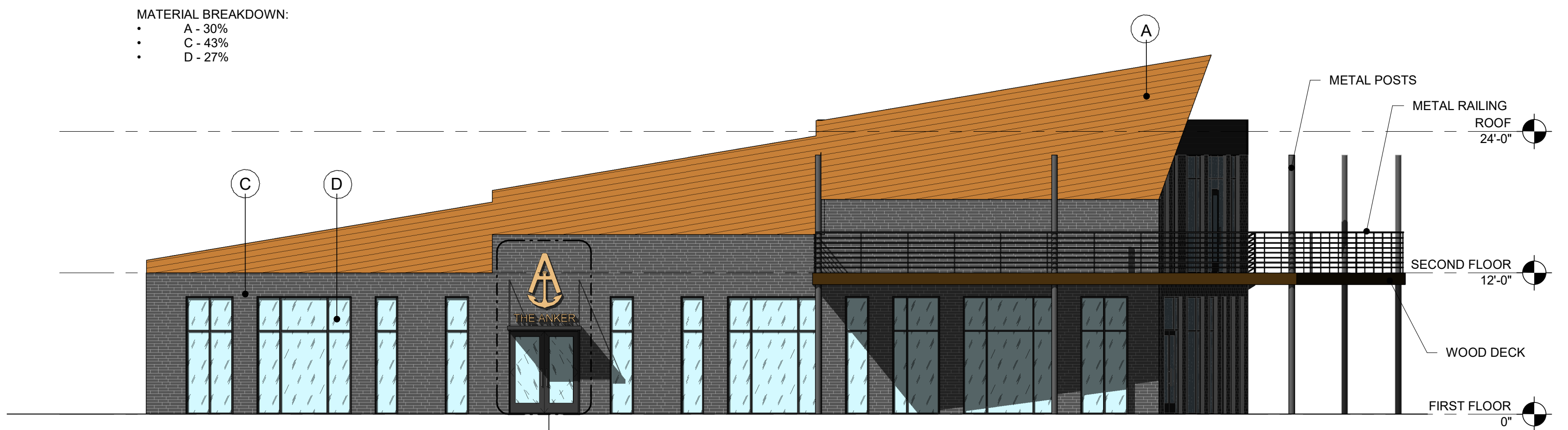
B1 EAST ELEVATION SCALE: 1/8" = 1'-0" MIN 50% PRIMARY MATERIALS
