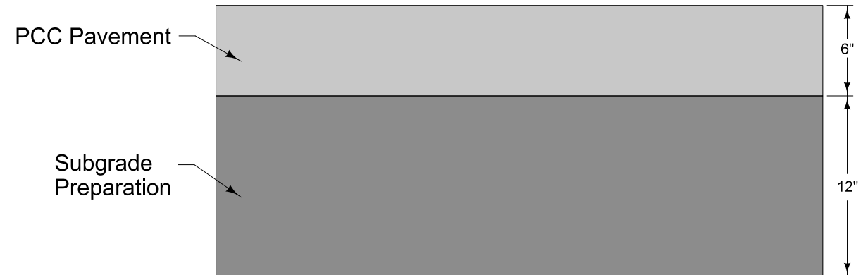
4 PAVEMENT TYPICAL NTS
